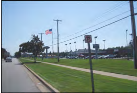
Access to adjoining parcels along Beacon Boulevard is fairly well managed with limited curb cuts and several shared points of access
