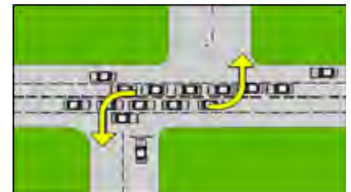
Ineffectively aligned opposing intersections create the potential for "left turn lock-up" situations
