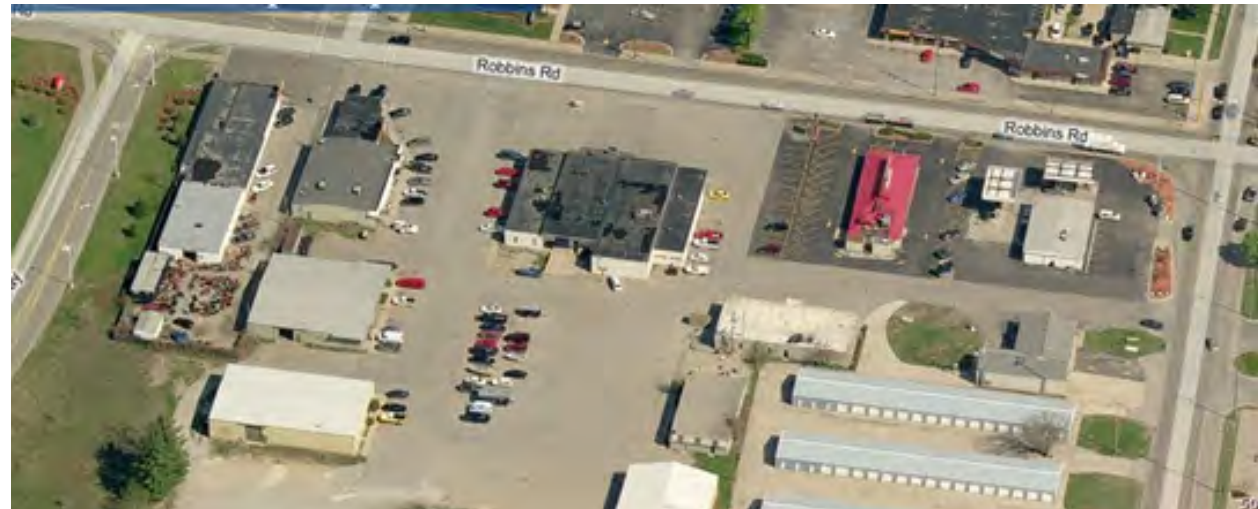
The lack of definition within the parking areas may lead to confusion for drivers and an unsafe environment for pedestrians.
